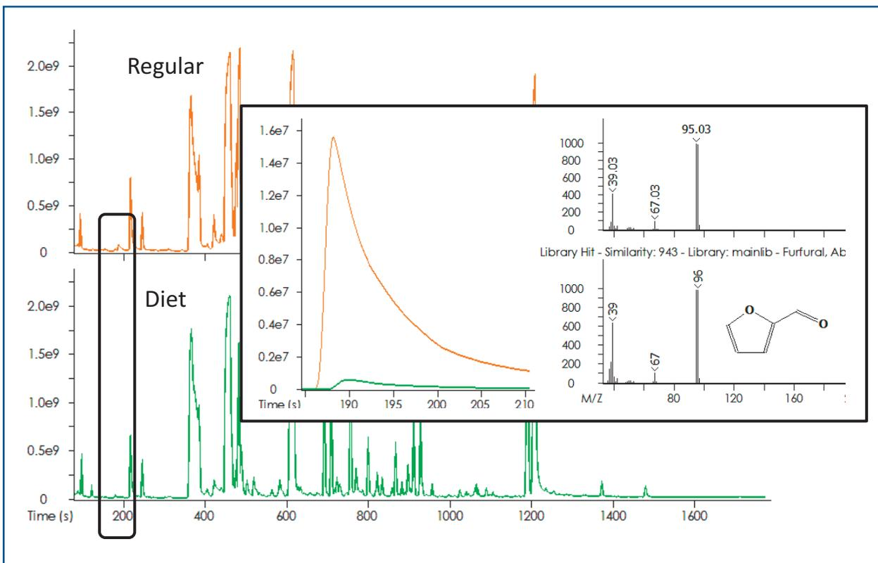
**Figure 4.** Taking advantage of all of the analytical capabilities of the Pegasus BT, differences between the diet and regular tea were observed. Here, furfural, a sugar degradation product, is observed in the regular tea, and at much higher levels than in the diet tea.
