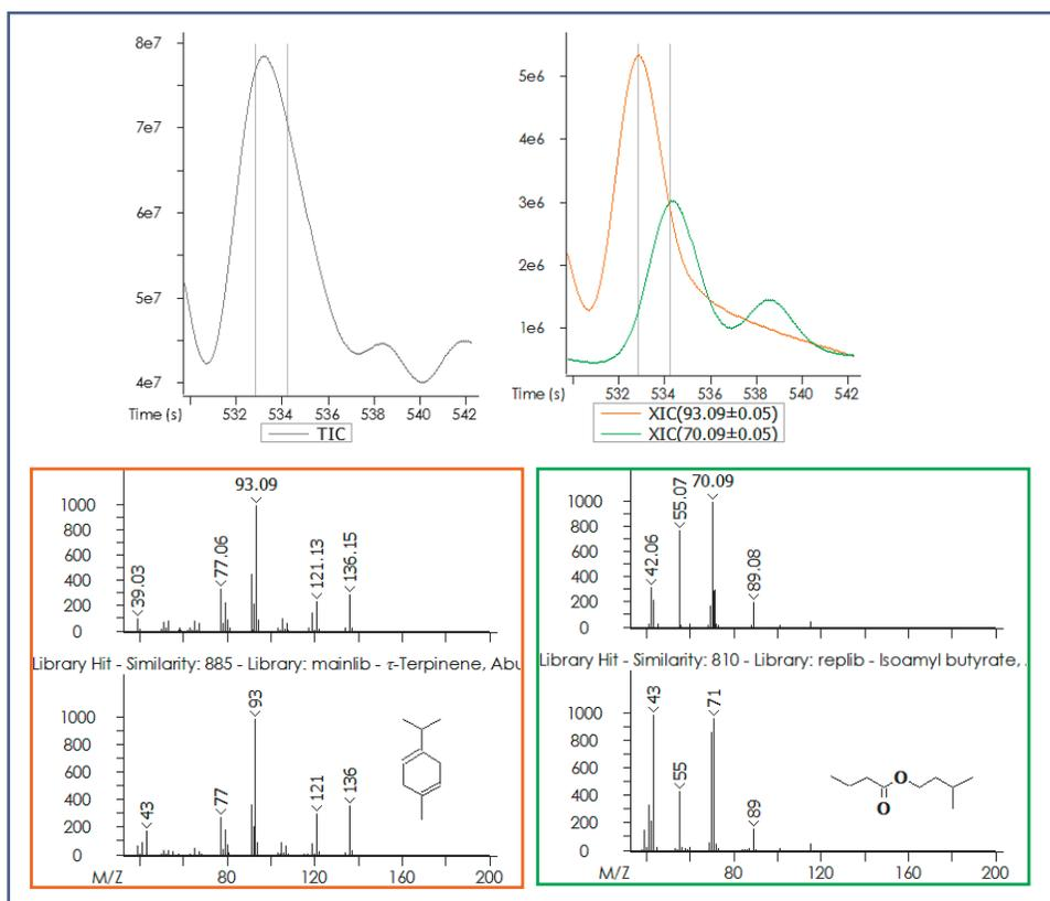
**Figure 2. Another case of deconvolution is shown from the diet fruit tea. In the TIC (gray), there appears to be only one peak, but by plotting XICs unique to each analyte, individual peak profiles were observed. Here, deconvolution mathematically resolved and tentatively identified gamma-terpinene, a terpene with woody, terpene, and herbal odor properties from isoamyl butyrate, an ester with fruity odor characteristics.**
